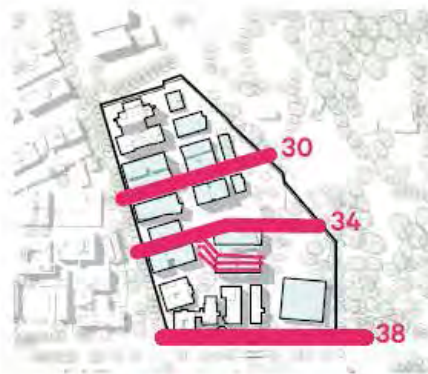
02 SITE BENCHING TERRACE STEPS
